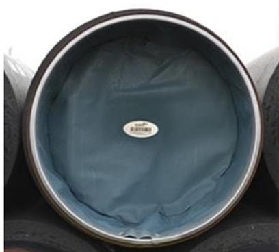
*Together with the producer of the tags, subsidiary company Dhatec has used a project to make sure that the Tags are attached to the end cap before they go to the coating sites. This way a protection product for our pipes becomes a ‘traceability tool’ as well.*
